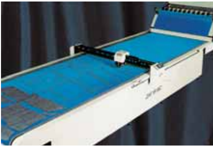
Continuous flow of material: Delivery, cutting discharge on a running conveyor belt.
